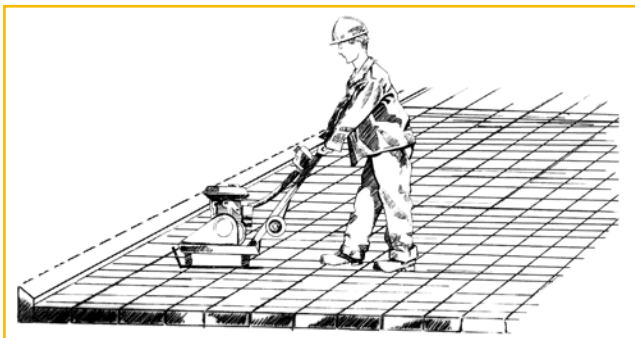
Figure 19: Vibrating the jointing sand into the joints
