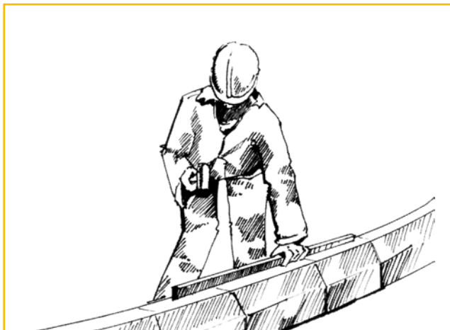
Figure 3: Checking of edge restraints
