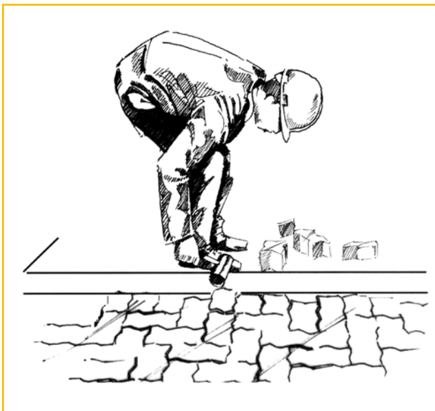
Figure 13: Fitting cut blocks into gaps
